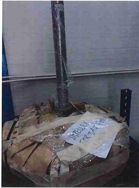
Impeller and shaft for JAZ fume exhaust fan
